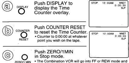
The Combination VCR will go into FF or REW mode and stop at the last point the Time Counter was set to 0:00:00.
