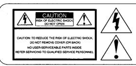
This symbol warns the user that uninsulated voltage within the unit may have sufficient magnitude to cause electric shock. Therefore, it is dangerous to make any kind of contact with any inside part of this unit.
